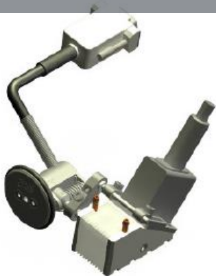
Motorized scanner installed on nozzle
